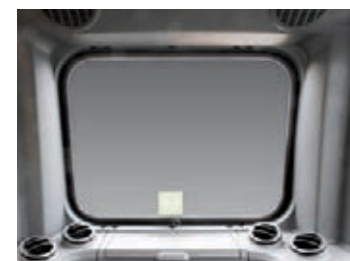
Rear Window Emergency Exit
