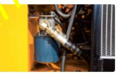
Remote Engine Oil Filter (HSL850-7A)
