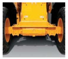
Enhanced axles improve driving on uneven ground conditions. Self adjusting brakes that automatically compensate disc wear, reduce service intervals and improve brake performance. The new load sensing hydraulic system with a variable volume piston pump and closed center main control valve, provide efficient hydraulic power and additional energy savings.
